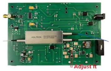
The device has a slightly difference  $V\pi$  for different operation frequency bands; therefore, adjustment can optimize the extinction ratio to some extent.
