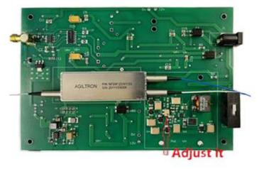
The device has a slightly difference Vp for different operation frequency bands; therefore, adjustment can optimize the extinction ratio to some extent.
